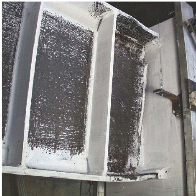
Figure D-90 Final condition of specimen NAI tested by Okazaki (2004)
