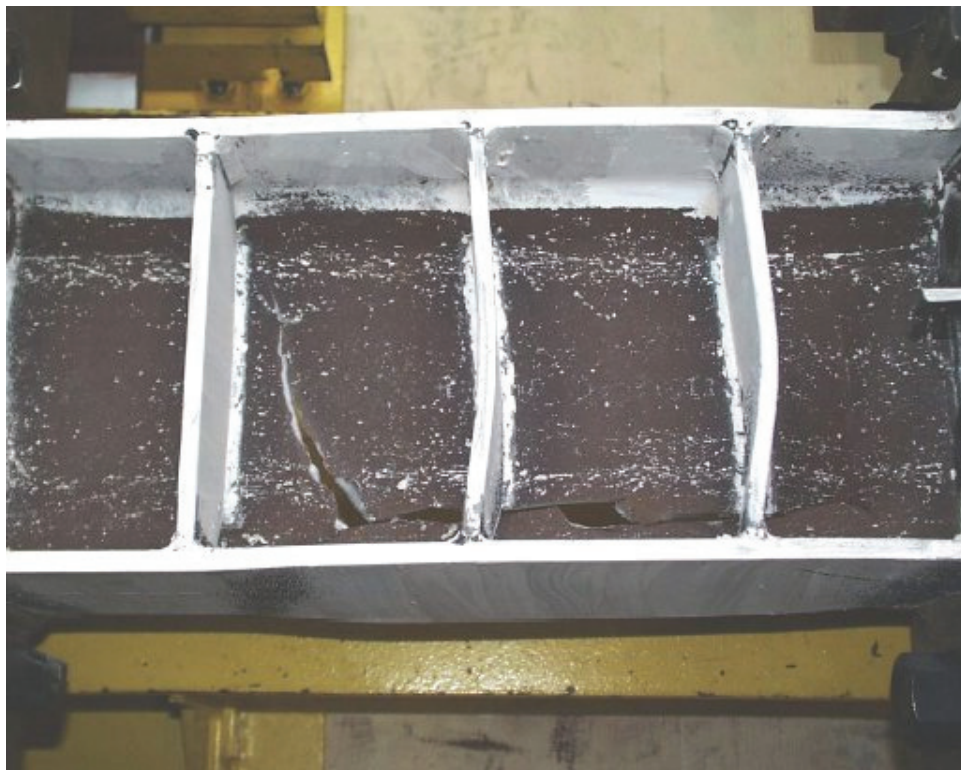
Figure D-56 Final condition of specimen 4A-RLP tested by Ryu (2005)
