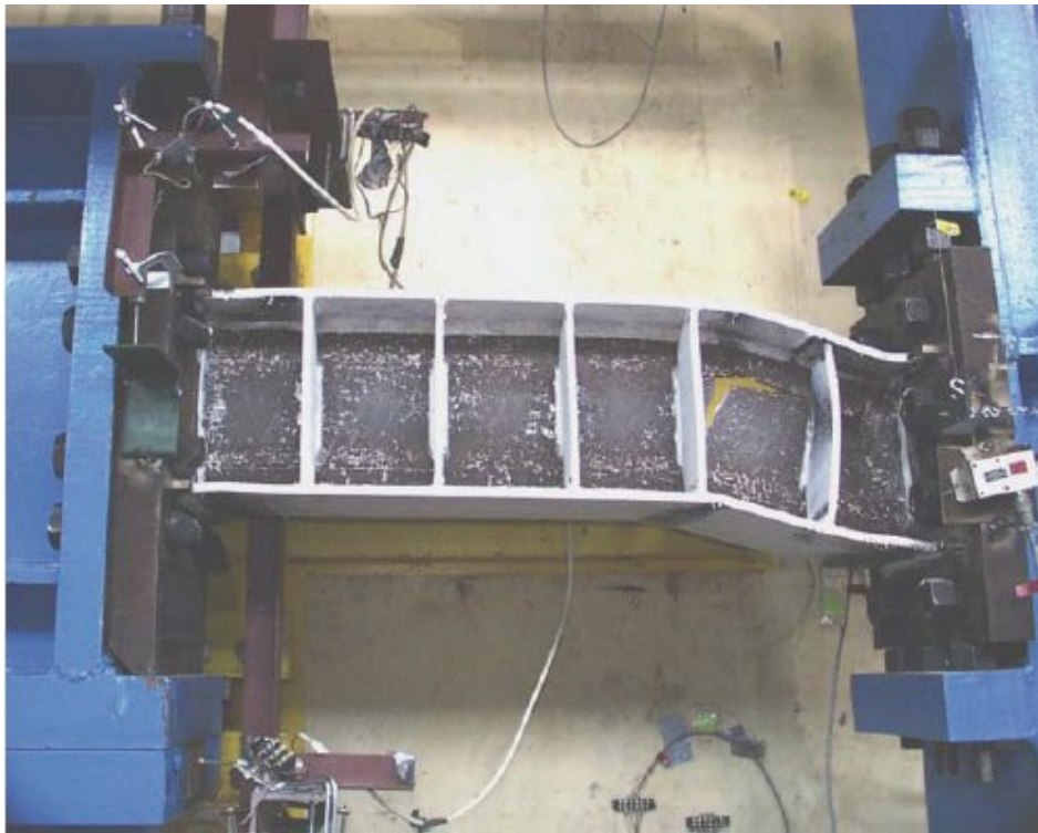
Figure D-96 Final condition of specimen 5 tested by Arce (2002)
