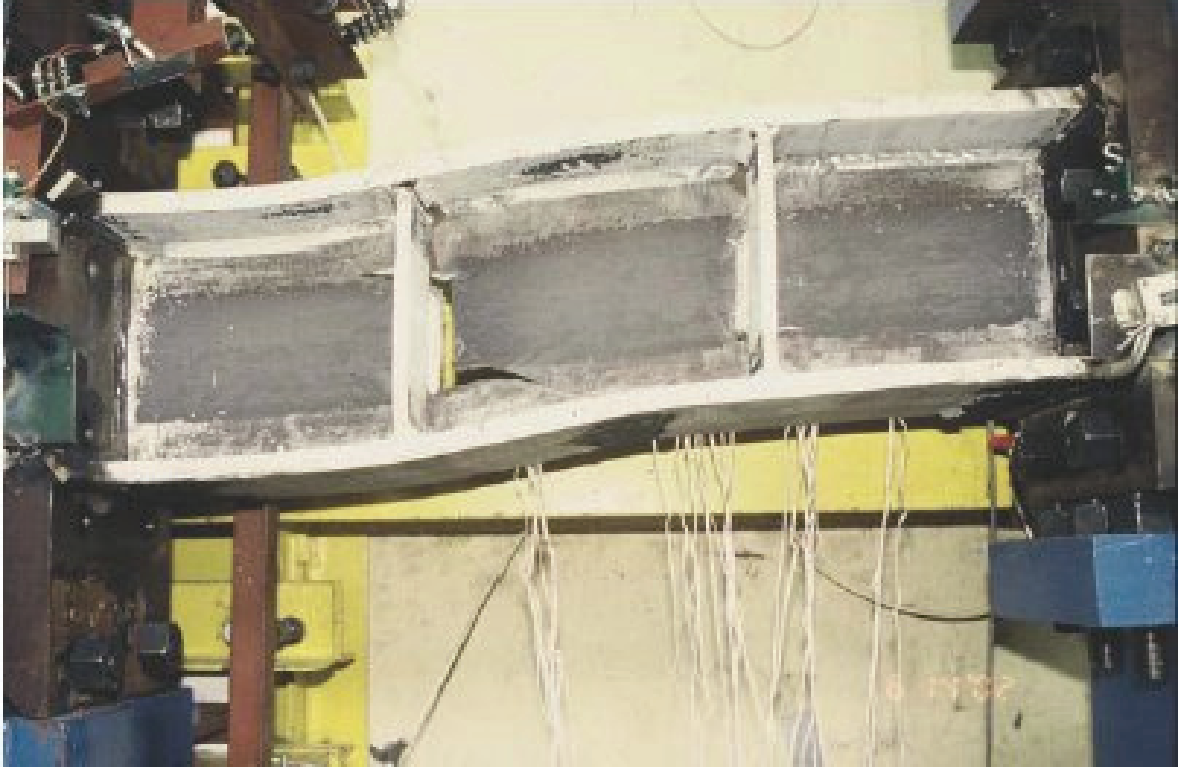
Figure D-45 Final condition of specimen 10 tested by Arce (2002)
