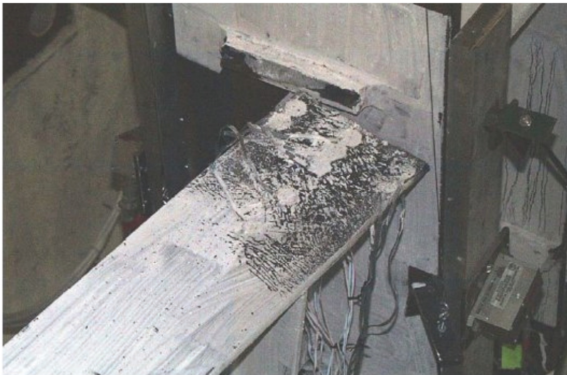
Figure D-85 Final condition of specimen MWI tested by Okazaki (2004)
