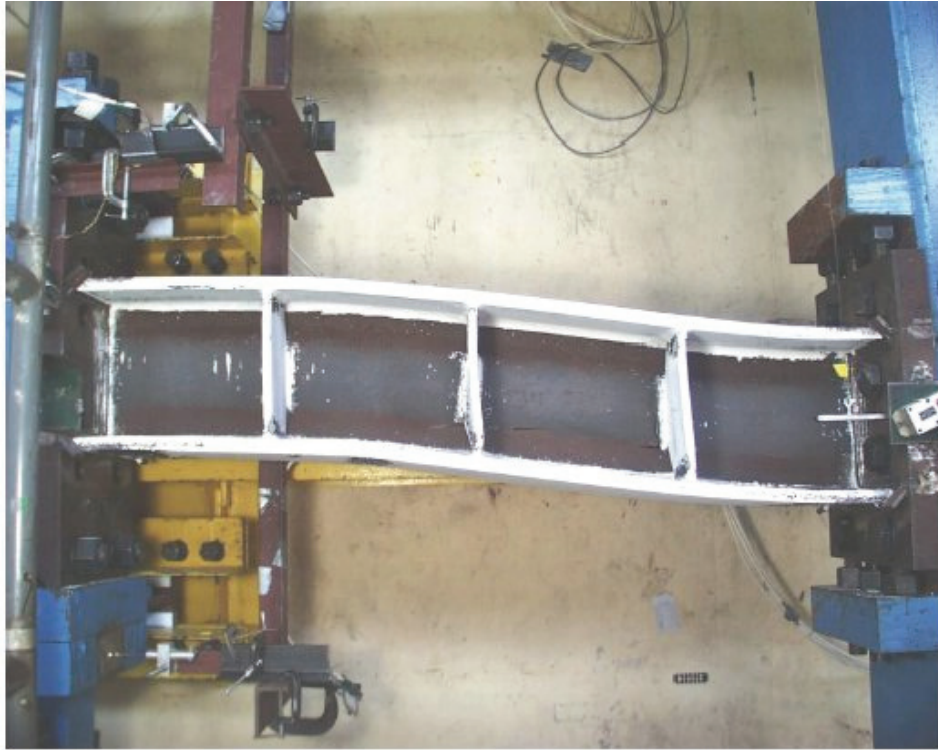
Figure D-101 Final condition of specimen 11-RLP tested by Ryu (2005)a
