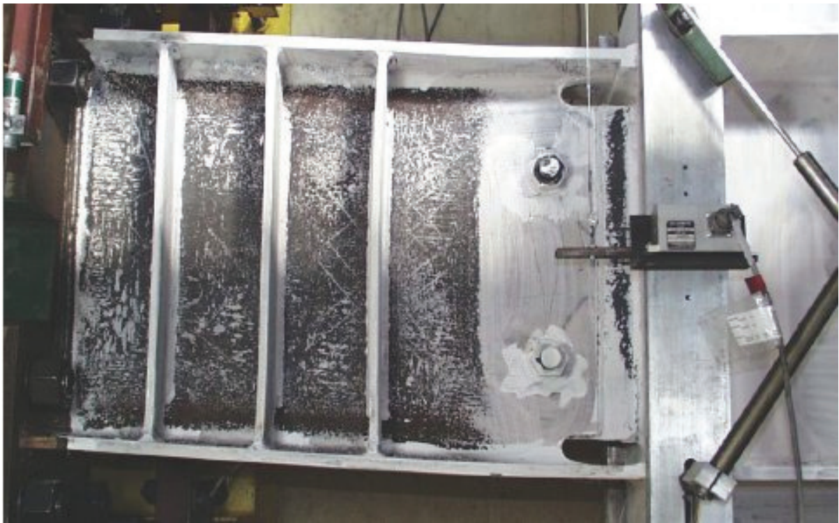
Figure D-36 Final condition of specimen FFS_RLP tested by Okazaki (2004)
