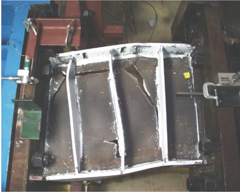
Figure D-61 Final condition of specimen 12-AISC tested by Ryu (2005)
