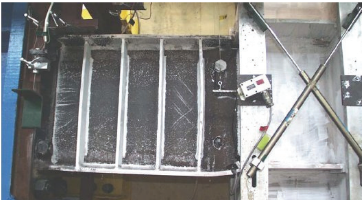
Figure D-33 Final condition of specimen PNS tested by Okazaki (2004)
