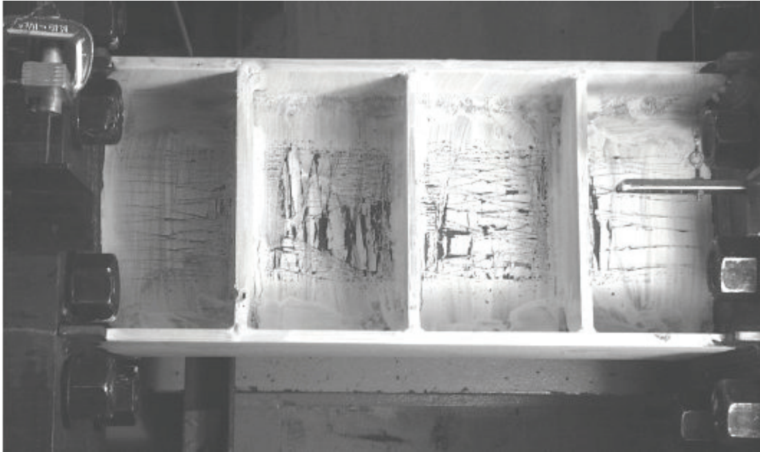
Figure 4-1 Web yielding on EBF link 2 tested by Galvez (2004)
