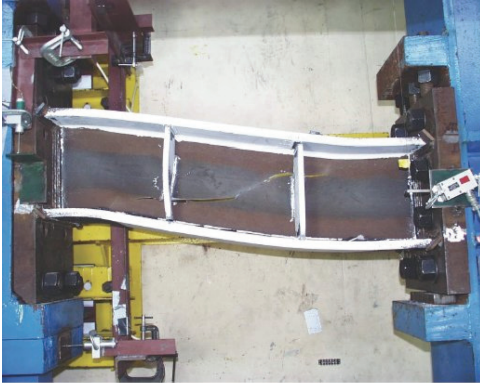
Figure D-59 Final condition of specimen 10-RLP tested by Ryu (2005)
