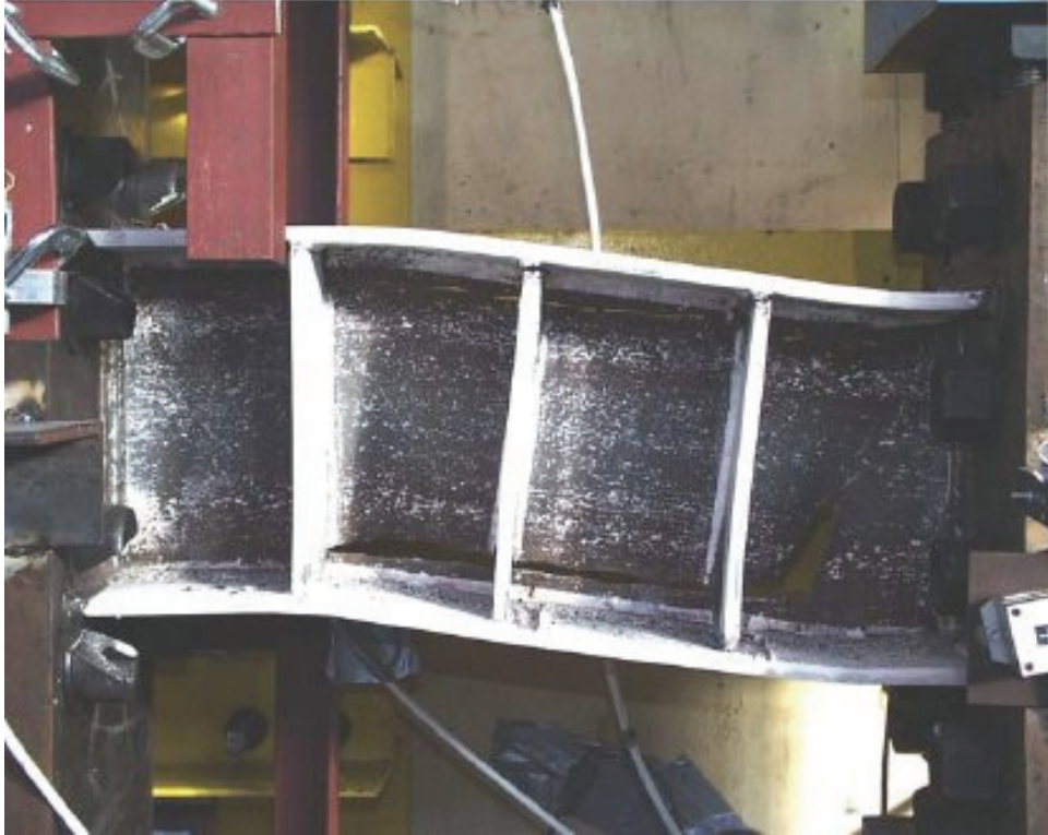
Figure D-41 Final condition of specimen 4a tested by Arce (2002)
