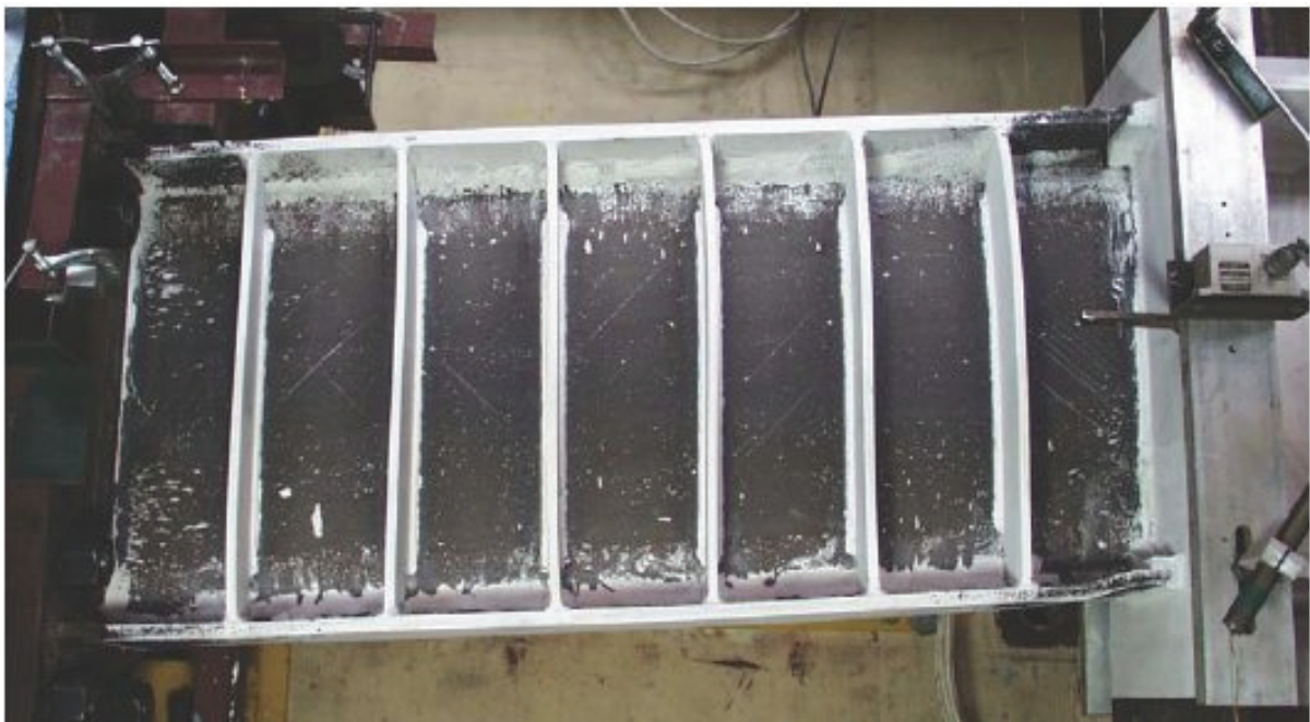
Figure D-38 Final condition of specimen NAS_RLP tested by Okazaki (2004)
