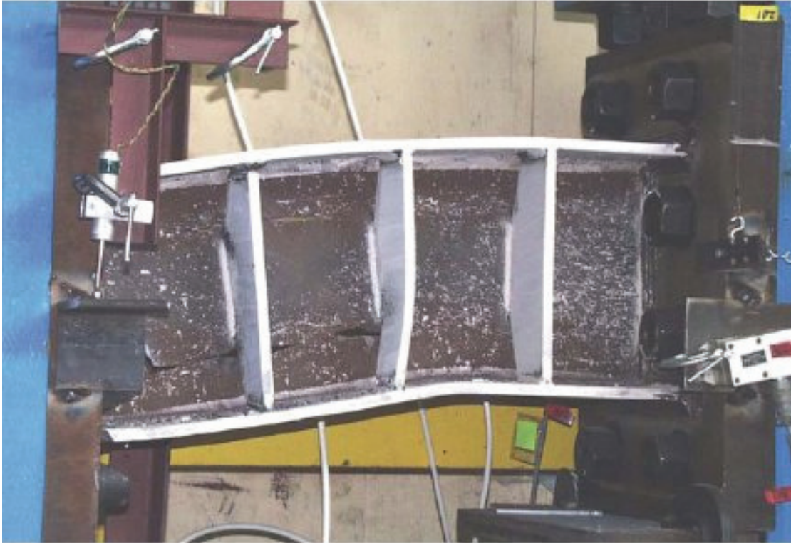
Figure D-43 Final condition of specimen 4c tested by Arce (2002)
