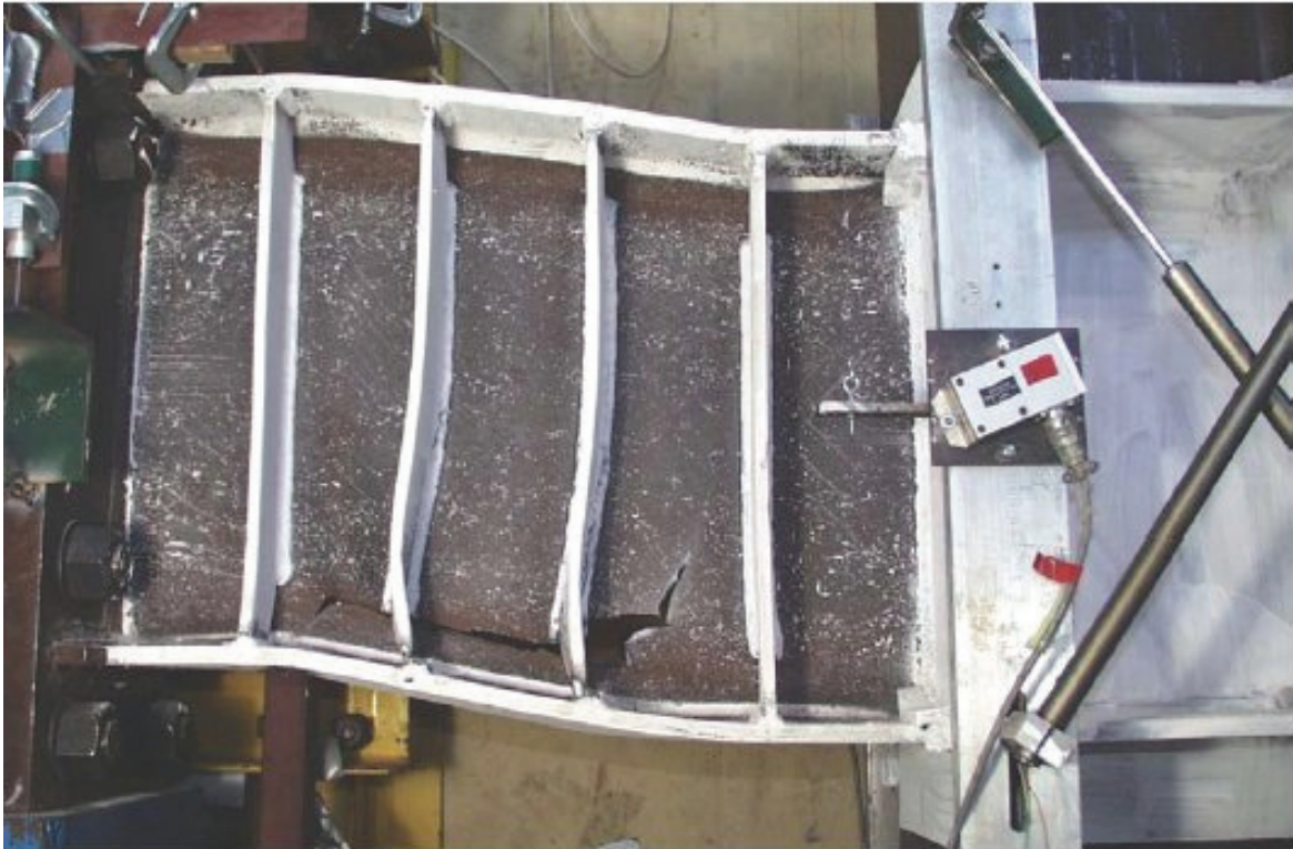
Figure D-37 Final condition of specimen NAS tested by Okazaki (2004)
