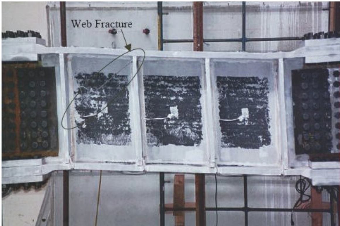
Figure D-39 Final condition of specimen Type 1 tested by McDaniel et al. (2002)
