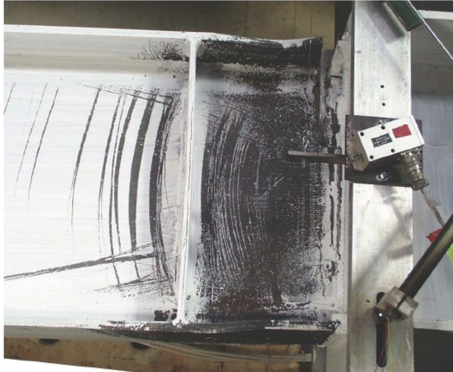
Figure D-91 Final condition of specimen NAM tested by Okazaki (2004)
