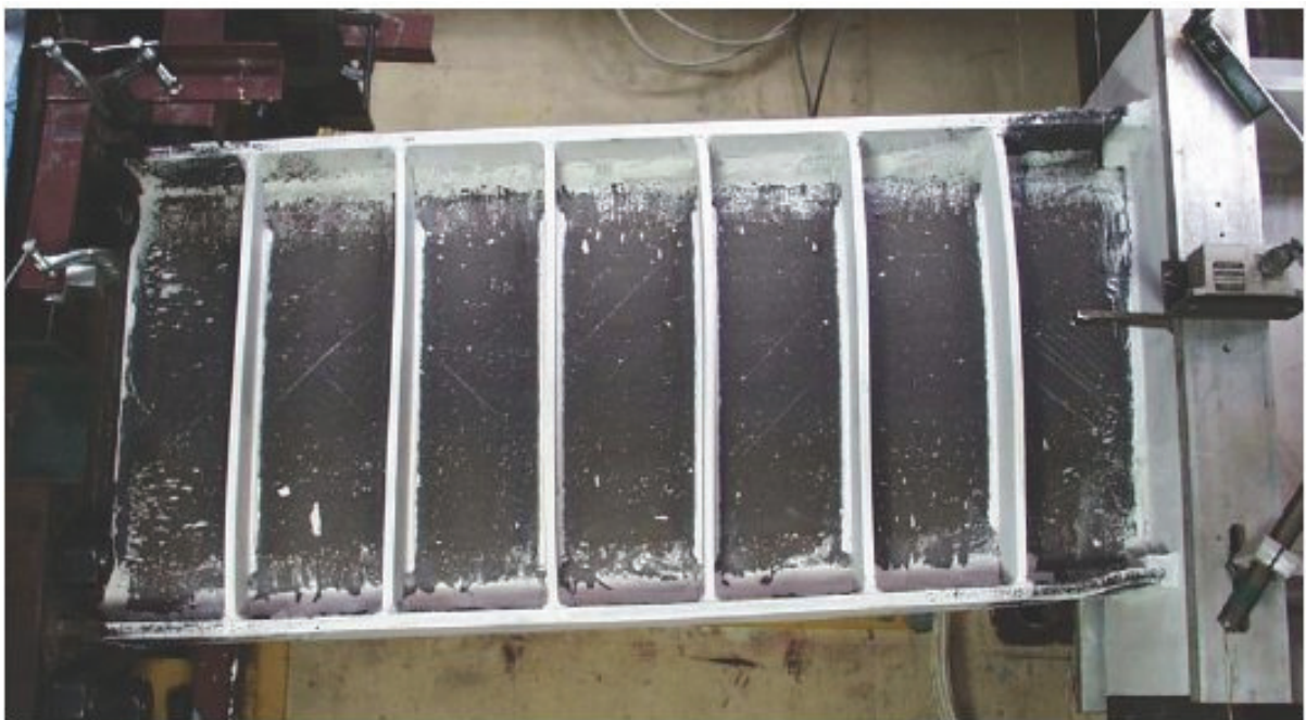
Figure D-92 Final condition of specimen NASL-RLP tested by Okazaki (2004)
